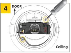
Secure the ceiling accessory to the ceiling using the provided screws and wingnuts.
