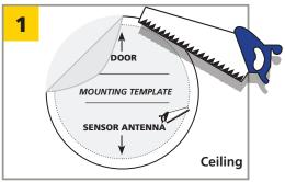
Place the mounting template in the desired mounting location and make the appropriate cuts.
