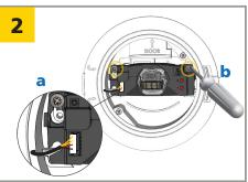
Route and connect the harness to the sensor, and then secure the sensor in the ceiling accessory.
