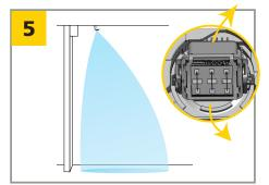
Make the appropriate radar adjustments to create the desired field shape and position. *Tilt angle should be 70° for optimal performance.*
