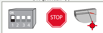
RELAY 1: STOP-impulse on swing side of door
