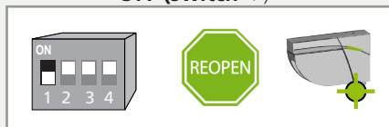
RELAY 2: REOPENING-impulse on approach side of door
