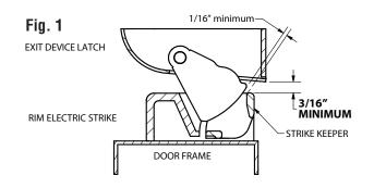
**NOTE:** Ensure a 1/16" [1.5mm] clearance between exit device <u>latch</u> and the electric strike <u>keeper</u> is maintained. Failing to do so will preload the strike and in turn will not allow the strike to release the door upon energizing. **WARNING:** For proper operation, a 3/16" gap (minimum) is required.
