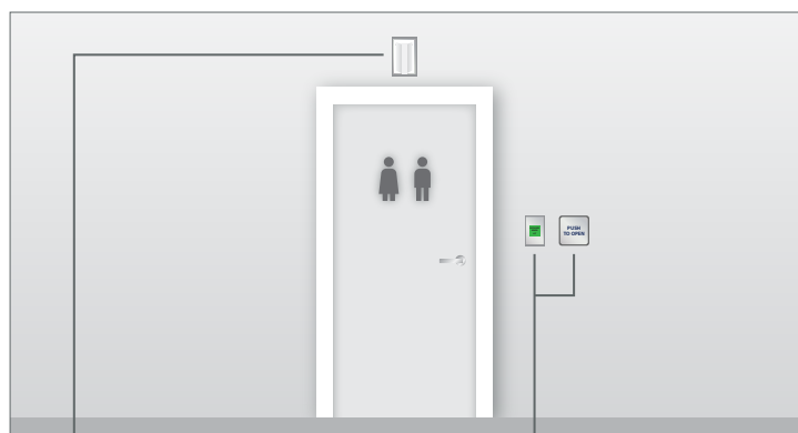
"ASSISTANCE REQUIRED" SIGNAL (LED + adjustable sounder) 10ARS
