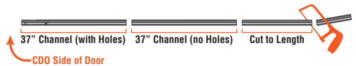
IMAGE 3: Cut and arrange the mounting channel sections
