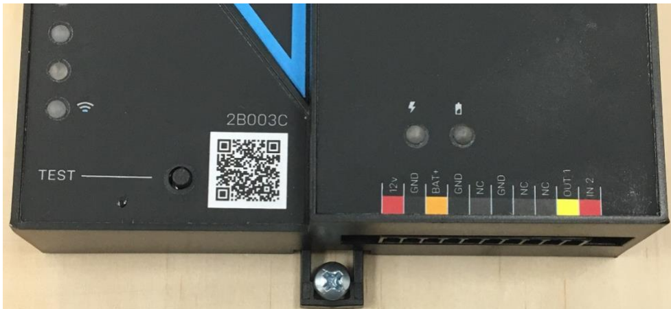
Figure 7: The bottom screw is shown mounted through the black DIN clip to the wall:
