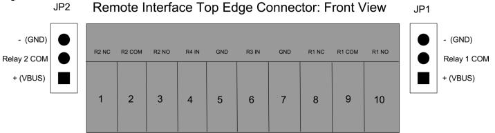
Figure 4: Diagram of Power Input, +VBUS, and JP1/JP2 functionality
