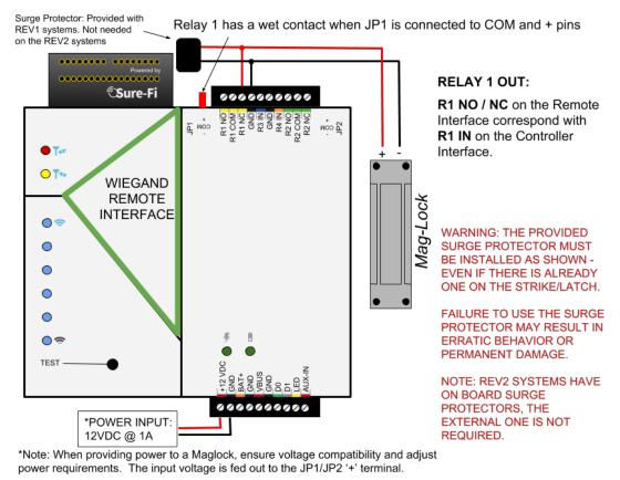
Figure 12: Wiring the Panel Door output relay to R1 IN & GND on the Controller Interface
