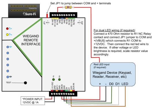
\*Note: When providing power to a wiegand device, ensure voltage compatibility and adjust power requirements. The Power Input voltage is fed out to the 'VBUS' terminal.
