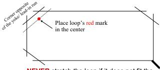
**NEVER** stretch the loop if it does not fit the groove, follow the instructions above and cut the corner opposite of the yoke.
