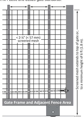
All openings of a horizontal slide gate are guarded or screened from the bottom of the gate to the top of the gate or to a minimum of 6 ft (1.8 m) above the ground to prevent a 2-1/4 inch (57 mm) diameter sphere from passing through the openings anywhere in the gate and in that portion of the adjacent fence that the gate covers in the open position.
