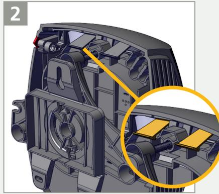
Pull the two legs on top in order to open the cover.
