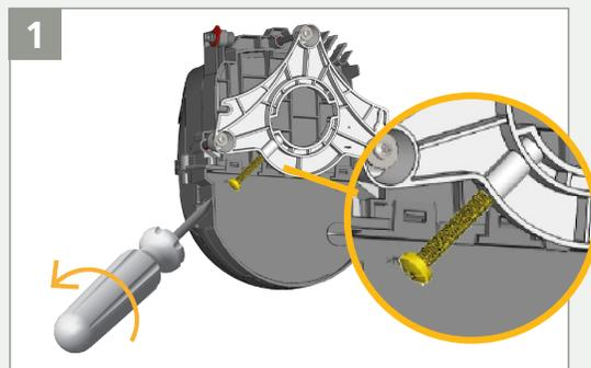
Verify that the angle lock screw is positioned as indicated. Unscrew slightly if necessary.
