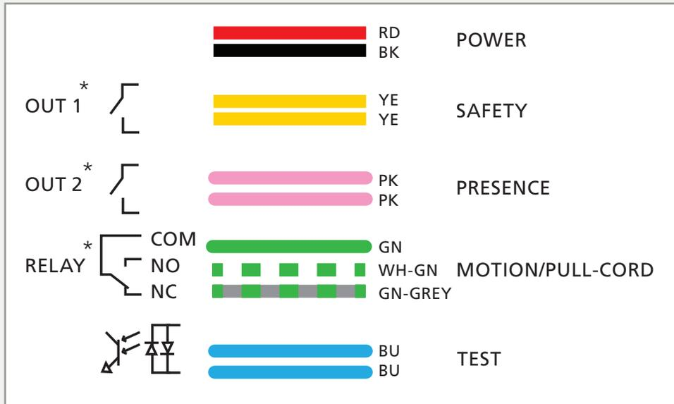
\*output status powered during non-detection with factory values
