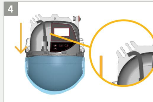
Plug in the connector and pass the cable (PN 35.1554) through the cable passage without making a loop.
