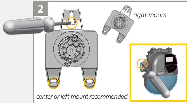
Remove the mounting bracket from the sensor by twisting CCW until the sensor detaches, and then secure the bracket to the wall. *If using a right-mount position, the bracket must be positioned at a ~30° angle.*
