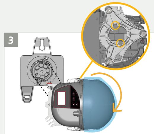
Tilt the sensor on its left side, align the tabs on the bracket with the notches on the back bracket of the sensor, and then rotate the sensor CW until the sensor is securely attached.
