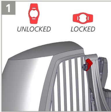
Before opening the sensor, make sure the cover is **not locked** (red cover lock). *Be sure to not turn the lock too far, because the lock can break.*
