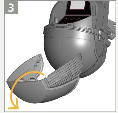
Remove the cover **completely** before installing the sensor.
