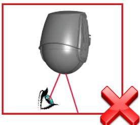
Do not look directly into the laser emitter or the visible red laser beams.
