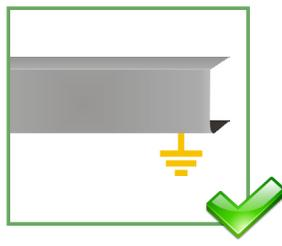
The door control unit and the header cover profile must be correctly grounded.
