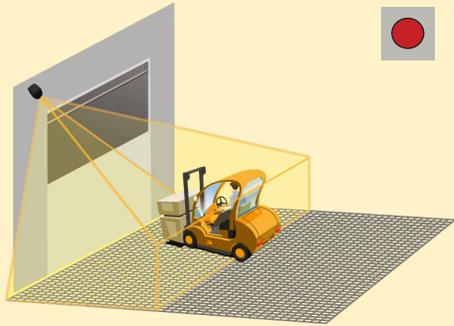
The presence field detects objects (moving or stationary) through the programmed field.
