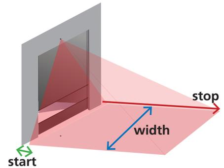
*For all three of the above parameters, the maximum reachable dimensions will automatically adapt according to mounting height.*
