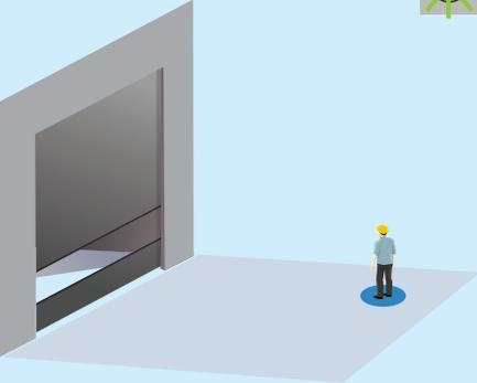
A virtual pull cord is a smaller detection zone that triggers the door to open when an object is present within it during a desired amount of time (minimum presence time).
