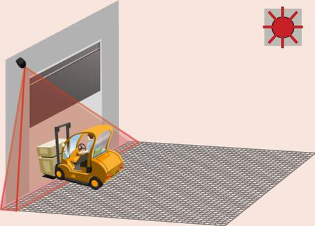
The safety field detects objects (moving or stationary) through the programmed field.
