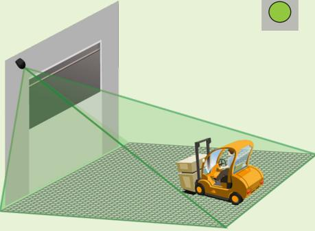
The motion field detects objects moving through the programmed field.
