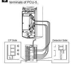
Connect the connector cable to the
