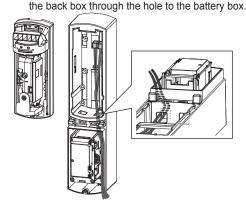
Adjust the wires so that they extend about 100 mm from the holes.
