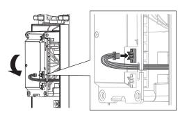
Route the three connectors of the back box through the slit on the upper part of the main unit of the receiver. For the transmitter, wire the two connectors in the same way.
