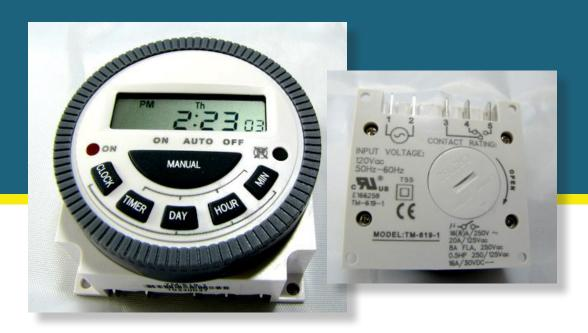
**The TM619 is a 7 day timer** that allows up to 8 on/off functions per day. It comes in 4 specific voltages: 12VDC, 24VAC/VDC, 120VAC and 240VAC. First, please check that you have the correct voltage for the application. The specified voltage is for the timer only. The output to your timed device goes through the contacts of the output relay which is rated to a maximum of 16a resistive and 8a inductive at 250VAC, 20 amps resistive at 125VAC and 16a at 30VDC.
