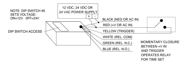
TIMEMATE: 12 VDC, 24 VDC OR 24 VAC ELECTRIC LOCK CONTROL
