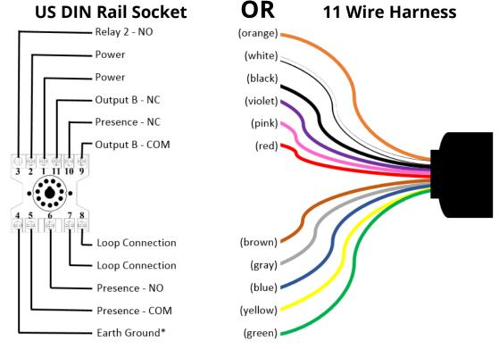
\*Must be connected to approved earth ground for surge protection to be effective
