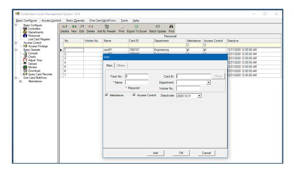
**Note:** The Card ID consists of the Facility Code + the Card ID, example 01300101 for facility code 13 and ID number 00101
