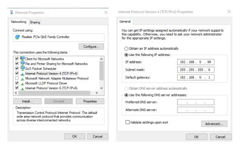
Above is an 'example' so remember your settings when you go to setting up the controller's address. Once you have this setup, you can close out the windows showing the information. Moving forward, you may have to shut down the firewall temporarily in order to add the network appliance. Note: You may also have to shut off your Wi-Fi on your computer.
