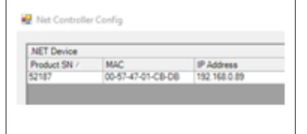
Select the 'Edit' ICON and enter you IP information for the controller, remember do not use the same IP address as your system. The 'example' is to set your IP address to 192.168.0.99 and then the controller could be set to 192.168.0.89. Now save your settings by selecting the 'Ok' ICON.
