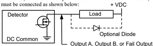
If the output is being used to turn on an inductive device such as a relay, a snubber diode should be wired in parallel with the relay coil.
